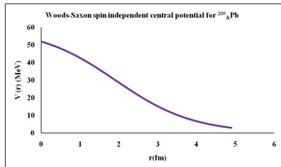
Fig. (2) Woods-Saxon spin independent central potential for  $^{209}_{\Lambda} \text{Pb}$
